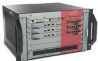
MC5000 Supports up to 1,500 access points Up to 20 Gbps encrypted throughput Headquarters, large campuses
